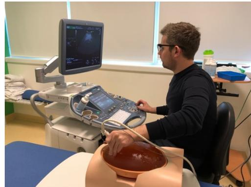
**Figure 2 – Experimental set-up of the Ultrasound Probe Tracker and the eye tracking glasses using a model abdomen.**
